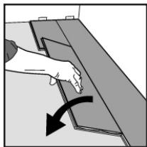
5. Install the boards in row 2 as instructed in Step 4. Place the next board tightly against the end of the previous board and drop it to lock it into place. If necessary, you can tap the board to fully lock it in.
