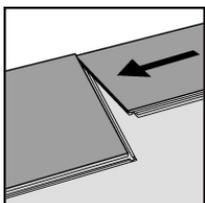
2. Place your second plank against the wall and drop the lip of the second plank onto the groove of the first plank. You should now have 2 planks tightly fitted together, both running along the same wall.
