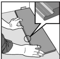
1. Place 3/8" wide spacers along the wall. Position the plank with the length of the board against the wall and the short end of the board against the spacer. You should have placed the board so that the groove sides are out and are showing. Allow a minimum gap of 3/8" (for subfloor movement or product expansion, which should be covered by moldings).
