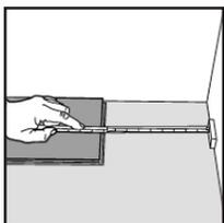
3. Continue laying planks end-to-end along the wall. When you get to the final plank, cut a board to fit leaving a 3/8" gap for expansion, and place a spacer between the plank and the wall.
